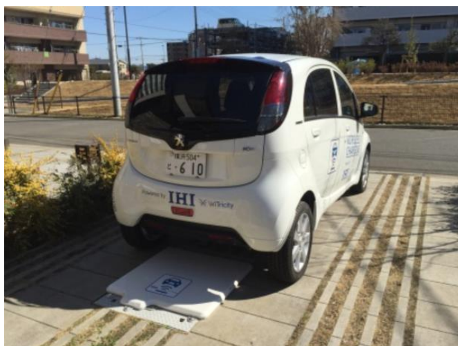
Figure 2. Prototype wireless charging pad under the car (Source: IHI).
